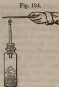
Simple mode of applying Marsh's Test.
